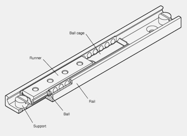
with runners connected in dual configuration (Full extension)
